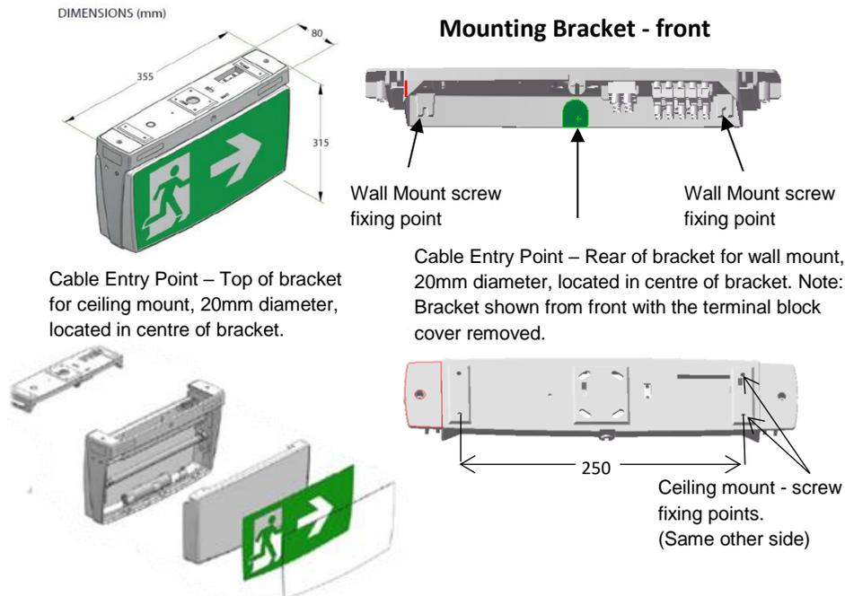
**Changing Exit Legend Inserts:** The Cleverfit Exit uses Clevertronics patented "Tamper proof" Exit legend cover and comes complete with spare legend inserts to enable straight on, left or right arrow as well as SS/DS combinations.
