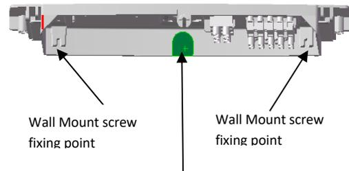
Cable Entry Point – Rear of bracket for wall mount, 20mm diameter, located in centre of bracket. Note: Bracket shown from front with the terminal block cover removed.
