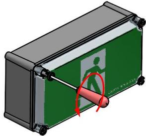
**Step 2** - Remove the Diffuser from the Cover
