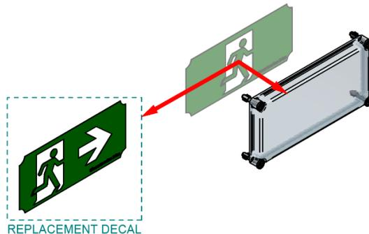
NOTE: Once Decals have been replaced, repeat 'Decal Replacement' steps in the reverse re-install the Cover, Diffuser & Decal
