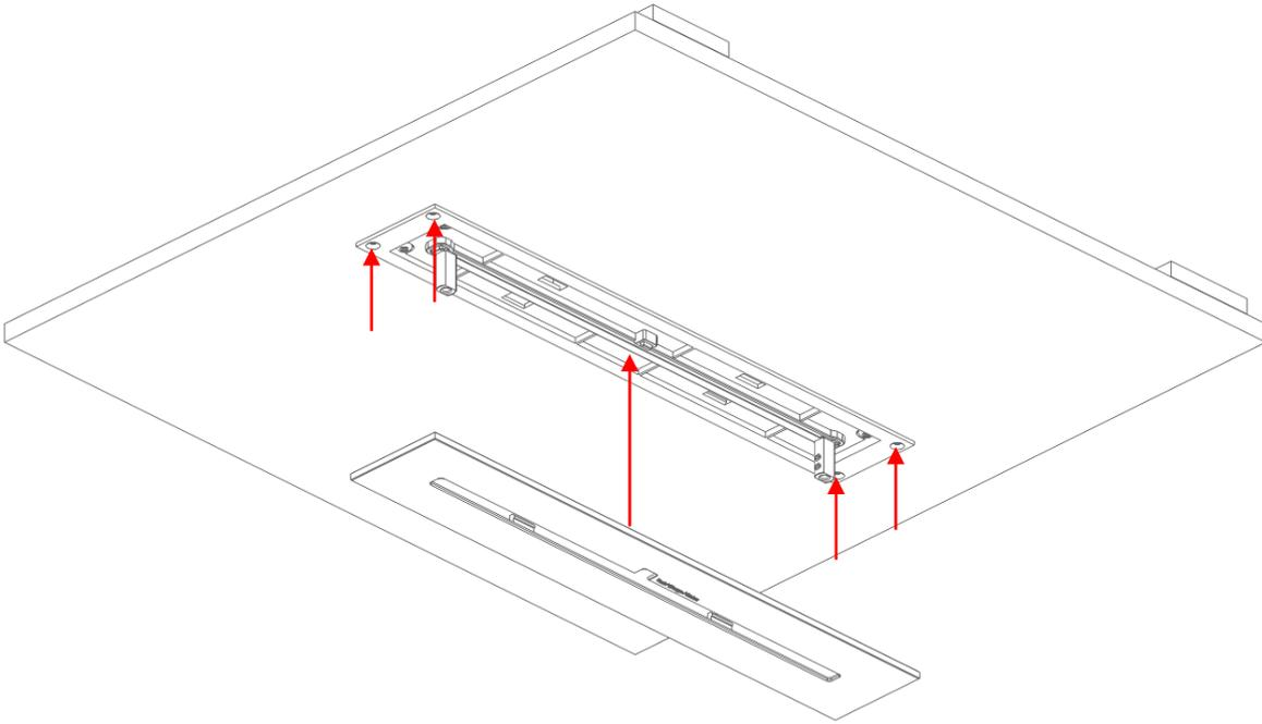
**Step 4** – Cut Rods to required length (Debur cut ends and remove any coating 10-12mm from rod end to provide electrical connection) and Insert Rod & Blade Assembly and tighten all grub screws.
