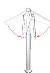
Compress Spring Toggle when inserting Adaptor Plate
