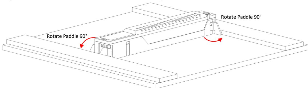
**Step 3** - Fix Top Assembly to the previously installed Timber Battens using appropriate fixings and install Cover Plate
