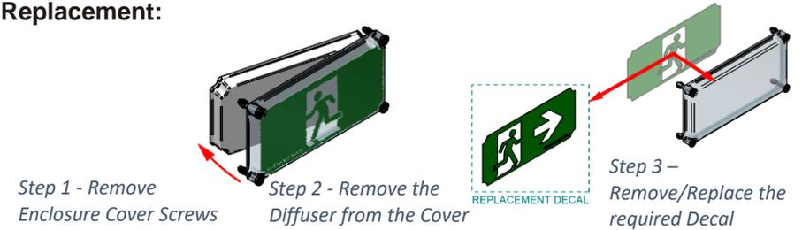
**NOTE:** Once Decals have been replaced, repeat 'Decal Replacement' steps in the reverse re-install the Cover, Diffuser & Decal
