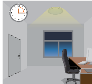
No area movement detected after time set at sensor
