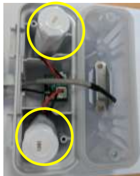
LED POD cover removed. Batteries highlighted
