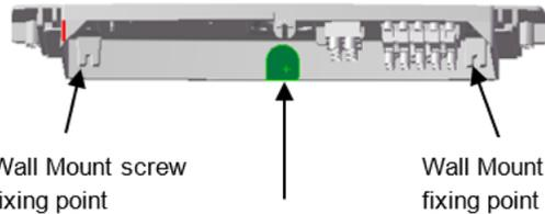
Cable Entry Point – Rear of bracket for wall mount, 20mm diameter, located in centre of bracket. Note: Bracket shown from front with the terminal block cover removed.
